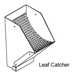
The Leaf Catcher designed to filter out small debris before causing problems in your perimeter drains. The self cleaning design is attractive and easily maintained at ground level.
