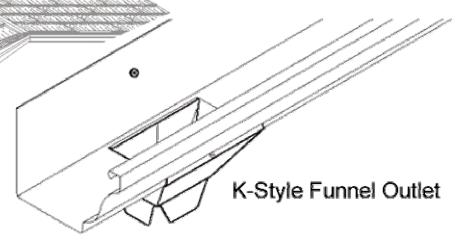
The large opening of the K Funnel style outlet allows for continuous flow and will not dam the opening like conventional plastic outlets.
